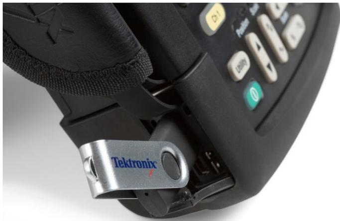
The standard USB ports facilitate data storage, data transfer, and instrument control
