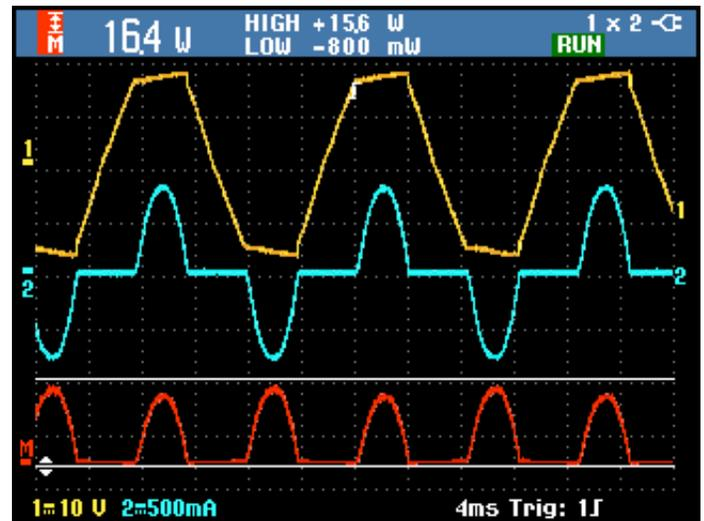
Easily calculate the instantaneous power by multiplying voltage and current waveforms
