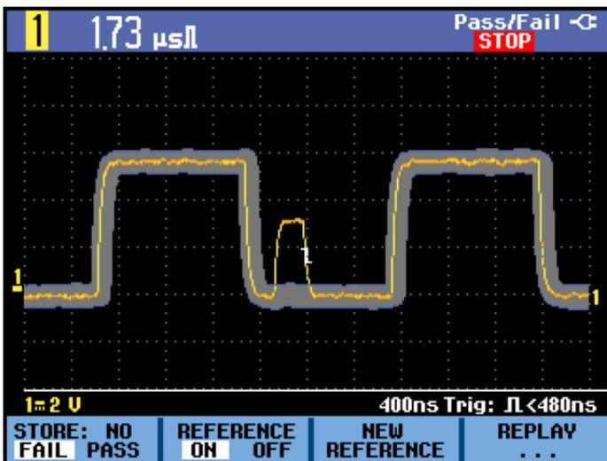
User-defined limit testing can easily identify random waveform anomalies
