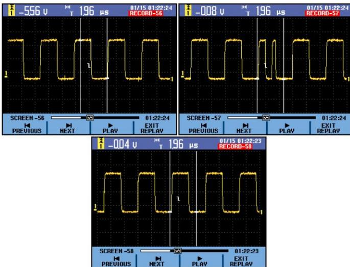
Playback of captured data is quick and easy with the THS3000 series oscilloscopes
