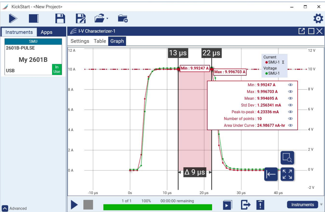
Figure 14: Analysis example of a pulse within KickStart.
