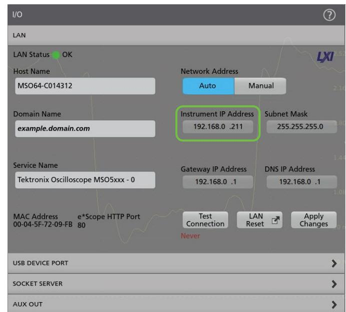
Figure 3. Example of the LAN Settings on a 6 Series MSO
