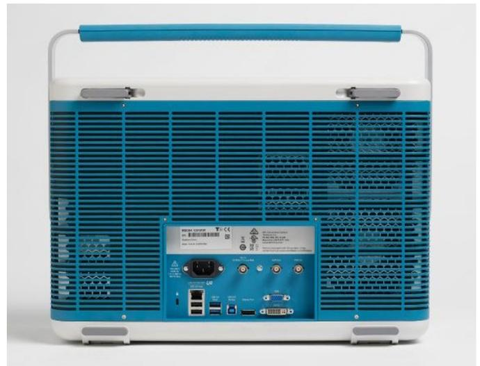
Figure 1. Many Tektronix oscilloscopes include USB and Ethernet LAN interfaces, such as this 6 Series MSO.
