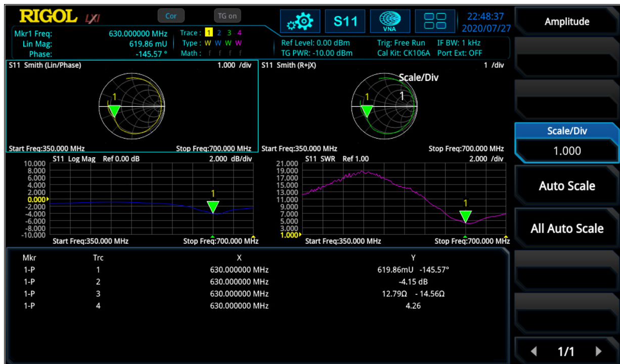
Figure 6: Different window of S_{11} parameter like smith- and Polar Plane, logarithm. Magnitude and SWR
