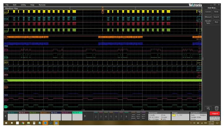
Figure 4. TekScope software uses the same user interface as the 4, 5 and 6 Series MSOs. The basic analysis package is free. With the premium Multiscope option it can collect data from two oscilloscopes at once.
