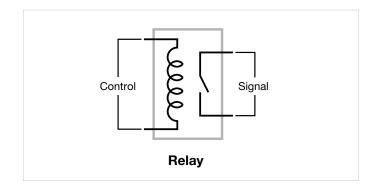
Figure 1. Simple electromechanical relay.
