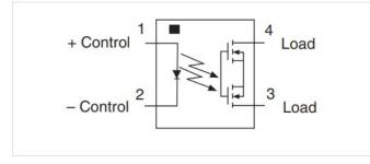
Figure 2. Simple solid-state relay.
