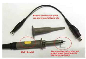
To reduce the effect of the probe in the vicinity of power by electromagnetic radiation, the following methods can use and reference
